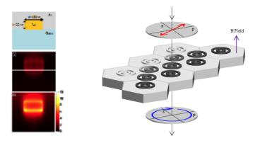
Figure: (left panel) electromagnetic field confinement effect due to the excitation of a localized plasmon in a metallic nanostructure; (central panel) example of a nanofotonic device for light polarization manipulation; (right panel) examples of ferromagnetic nanoscale optical objects implementing magnetoplasmonic functionalitites.
